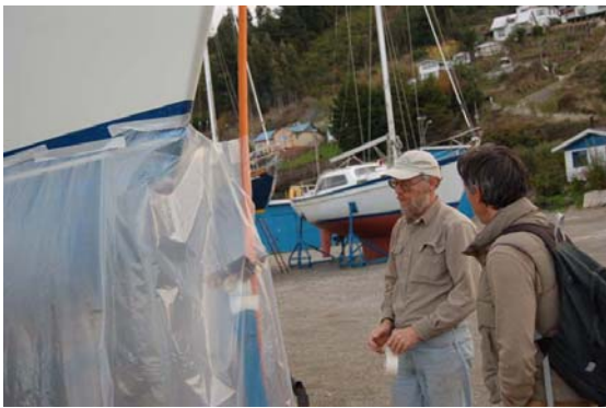
To keep the heat in a plastic tent was set up for the epoxy to cure. David Masters and Claude Gosselin also helped patch up Red Thread's underside.
