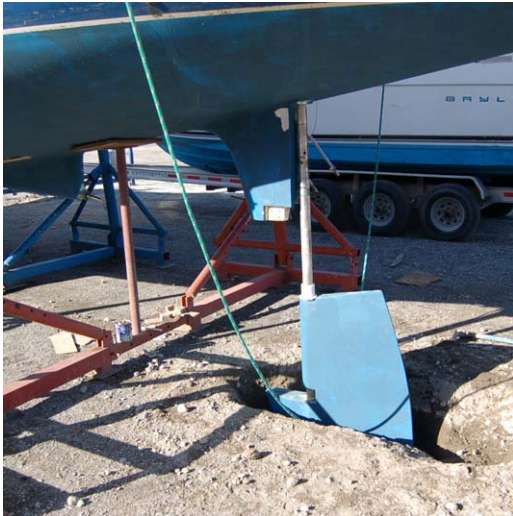
The rudder had to be removed for repair. The bottom 6 inches were torn off by the rocks, but the boat sailed all the way to port despite the damage.
