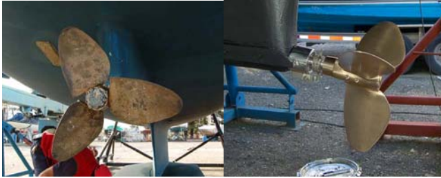
Before and after propeller notice on the left the upper blade turned wrong way. Cutters were added to the new propeller.
